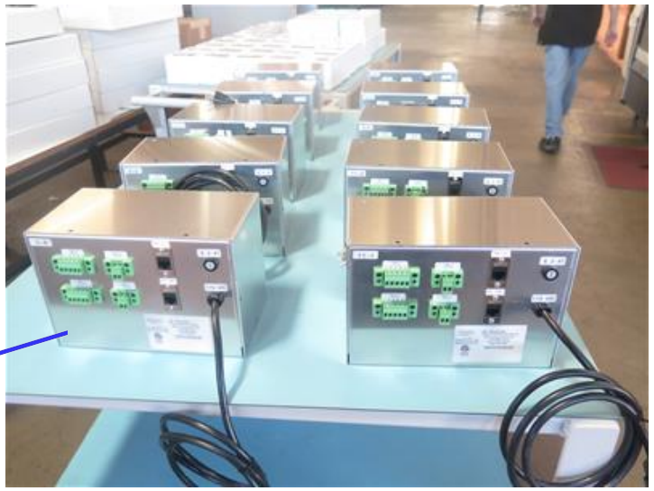
LED drivers being assembled and tested in the City Theatrical's Electronic Assembly room.
