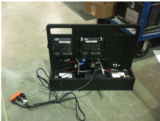
This is a shot of one of the SHoW DMXReceiver/Dimmer/Battery/Autocharger sleds made for the production by Scenic Solutions LLC of Dayton OH - http://www.scenicsolutions.com/ - Dan McLaughlin and his staff built all of the dimming and control gear for the scenic mounts into sleds like this. The sled hangs on the scenery walls by the handle holes and can disconnect and slide into purpose-built crates for traveling. There are relays built into it so that the batteries will charge when plugged in to line voltage and the batteries will not discharge when line voltage is disconnected, except for when they're in use.
