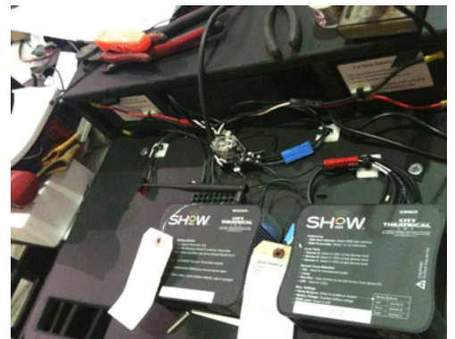
You see a close-up of the SHoW DMX Receiver/Dimmer/Battery/Autocharger sled here with detail of the terminal block, relay and connections
