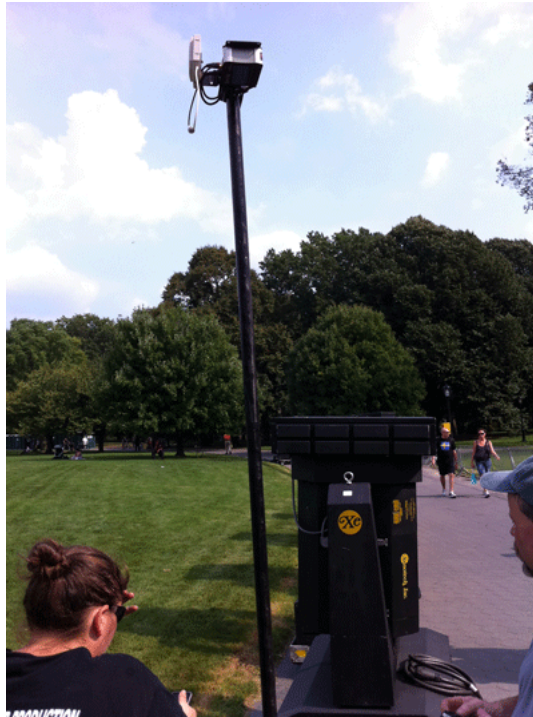
A example of good antenna placement. This is a focussed panel antenna placed high above the heads of the crowd with line of sight to the Transmitter.
