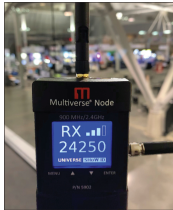
↑ At a distance of approx. 500ft, I had good signal strength using the 2.4GHz band in a crowded space
