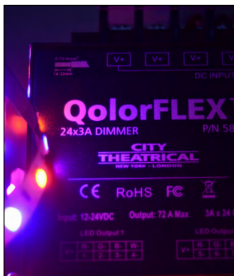
QolorFLEX 24x3A Dimmer shown controlling QolorFLEX LED Tape (left) and QolorFLEX® NuNeon (right).
