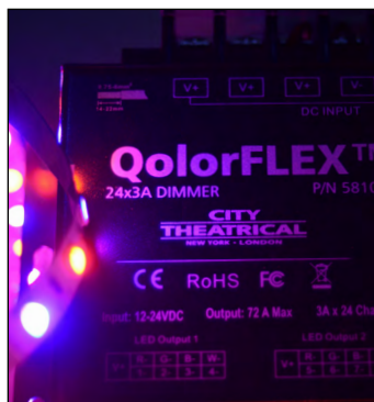
QolorFLEX 24x3A Dimmer shown controlling QolorFLEX LED Tape (left) and QolorFLEX® NuNeon (right).
