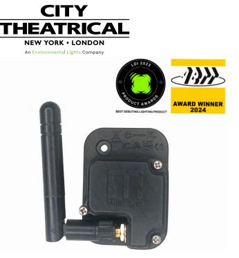
**Multiverse Connect Module, 2.4GHz** (P/N 5914) is a small device that brings all the capabilities of Multiverse wireless DMX/RDM on the 2.4GHz band to a lighting fixture built by an OEM manufacturing partner of City Theatrical, such that the fixture has a Universal Connect Module socket built into it. The chassis of the device plugs into the fixture, and with a few menu changes on your fixture, it becomes wireless.
