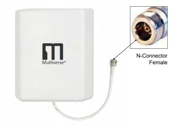
The **7dBi/8dBi Panel Antenna, 900MHz/2.4GHz, Dual Band** (P/N 5981) is a broadband, low VSWR, directional antenna with a 60° Beam spread. While it is designed for for outdoor reception, it can be used for indoor or outdoor projects.
