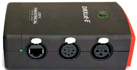
DMXcat-E hardware, side view
