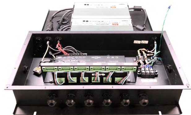
Custom low voltage QolorFLEX LED Dimmer enclosures
