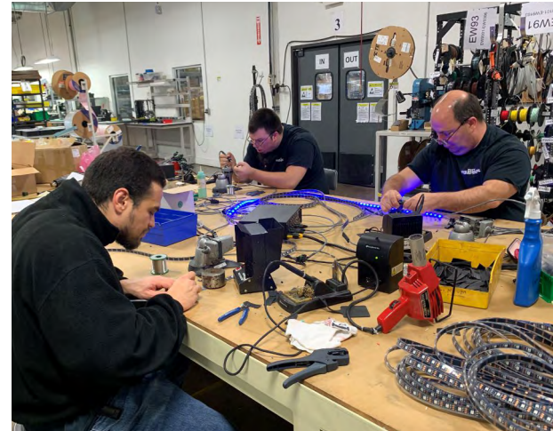
Custom cutting QolorFLEX LED Tapes, QolorFLEX NuNeon, and QolorPIX Pixel Tape
