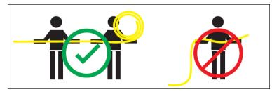
Only bend the neon in its intended direction. Do not twist or stretch neon. Above image shows horizontal bending neon.
