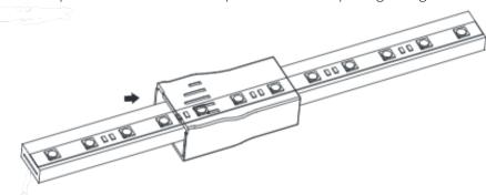
2. Unfold the metal clip and then install the metal clip onto the strip ensuring that it lines up with the edge of the strip.
