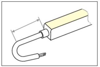
Leave 20mm of cable extended from the connector before bending.
