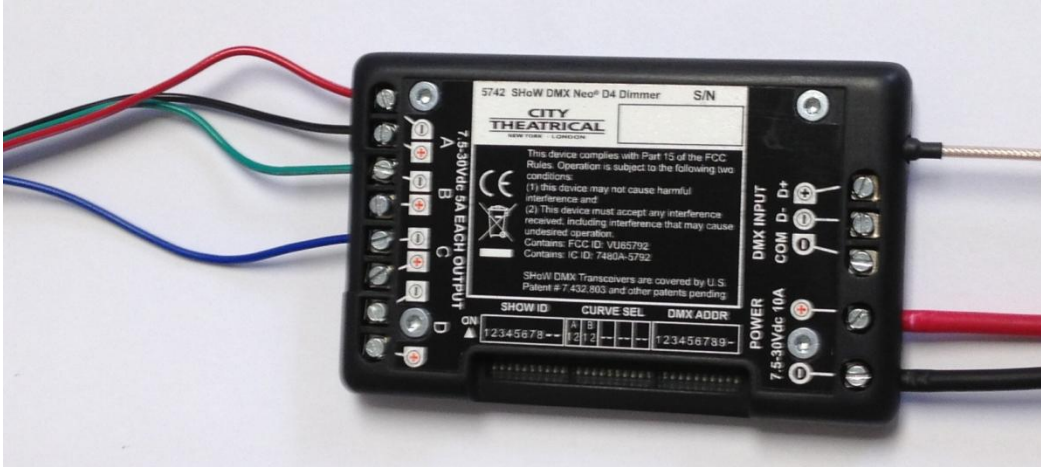
D4 Dimmer connected to RGB Tape
