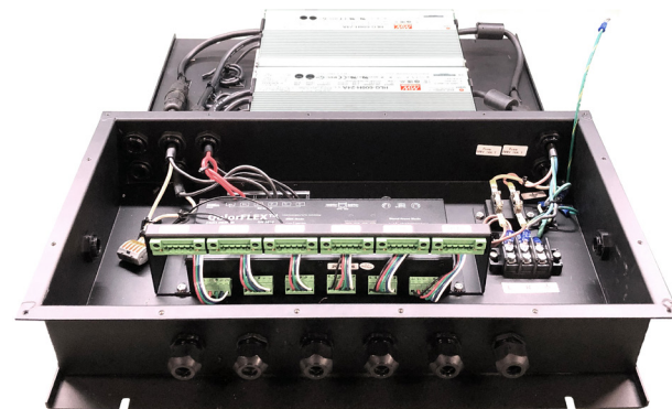
Custom low voltage QolorFLEX Dimmer boxes
