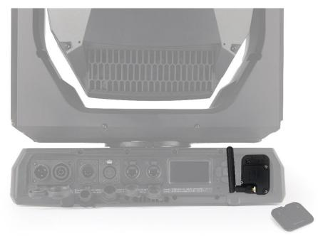
City Theatrical's new Multiverse Connect Module is a small device that brings all the capabilities of Multiverse wireless DMX/RDM to a lighting fixture built by an OEM manufacturing partner of City Theatrical, such that the fixture has a Multiverse plug built into it.
