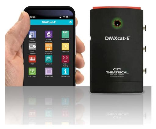
City Theatrical's new DMXcat-E (P/N 6100) allows users to view and send Ethernet protocols, including sACN and Art-Net, as well as PoE voltages, as well as perform cable testing of 5-pin XLR and RJ45 cables, and display SMPTE LTC and MIDI.
