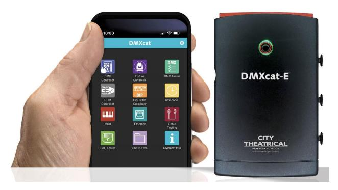
When connected to the new DMXcat-E™ device, City Theatrical's DMXcat® smartphone app shows new applications including: Timecode, MIDI, Ethernet, Cable Testing, and PoE Tester.
