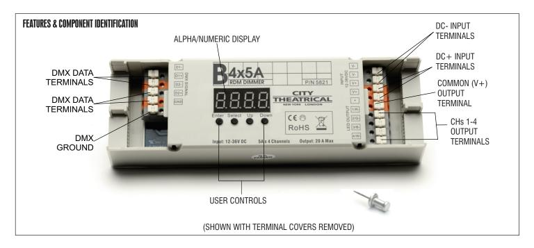
The B4 x 5A RDM Dimmer can control a full 20A of LED tape spread over four channels of 5A each. It uses constant voltage technology which ensures consistent full range dimming that is especially important at low end light levels. The unit is easily surface mounted and has terminal blocks for all electrical and data connections.
