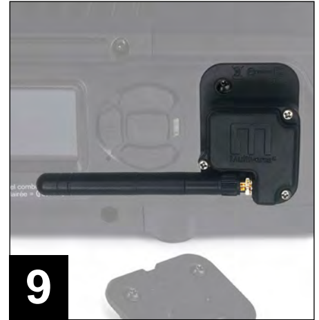
9. Once secured, the Multiverse Connect Module installation is complete.
