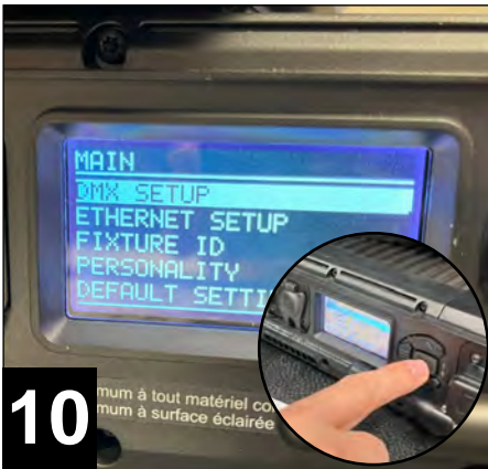
10. Click the buttons to the right of the fixture's screen, to find "DMX Setup" under the Main navigation. Navigate to the two sub-menus required for setup: "Wireless" and "DMX Universe."
