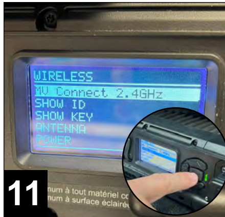
11. In the "Wireless" menu, the fixture will auto-detect if it is connected to a Multiverse Connect Module.
