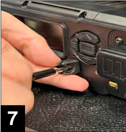
7. Fasten the antenna clip to the fixture base, which will hold the antenna in place.
