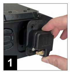
1. Plug the Multiverse Connect Module into the fixture base.
