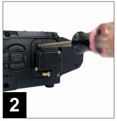
2. Screw the Multiverse Connect Module onto the fixture using a Phillips Head screwdriver and the screws that come with the fixture.
