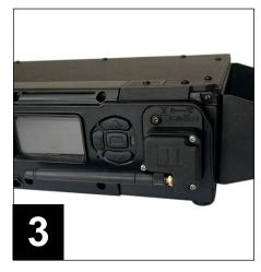
3. Attach the 2.4GHz antenna to the Multiverse Connect Module, and you're ready to use wireless DMX/RDM with the fixture!
