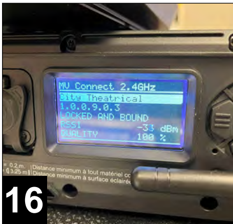
16. Access the “Module Name” menu to view additional information, including: City Theatrical manufacturer name, firmware version, locked and bound status, and signal strength and quality.
