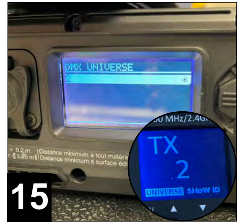
15. Navigate to the “DMX Universe” menu to confirm the selected universe matches the Multiverse Node, or other wireless DMX transceiver. In this example, Universe should equal 2 (refer to step 3).
