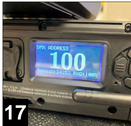
17. The fixture’s outermost menu will indicate in “DMX Address” whether it is receiving wireless DMX from the Multiverse Connect Module. It displays the SHoW ID and quality as a percentage.
